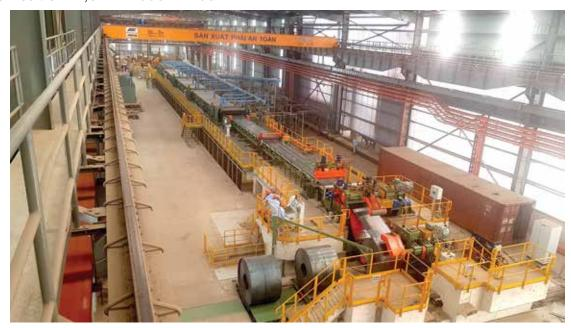
The Cold-rolling Machine, Continuous Galvanizing Line and Continuous Color Coating Line are fully automated, ensuring millimeter accuracy over each 10,000 m2 surface.
